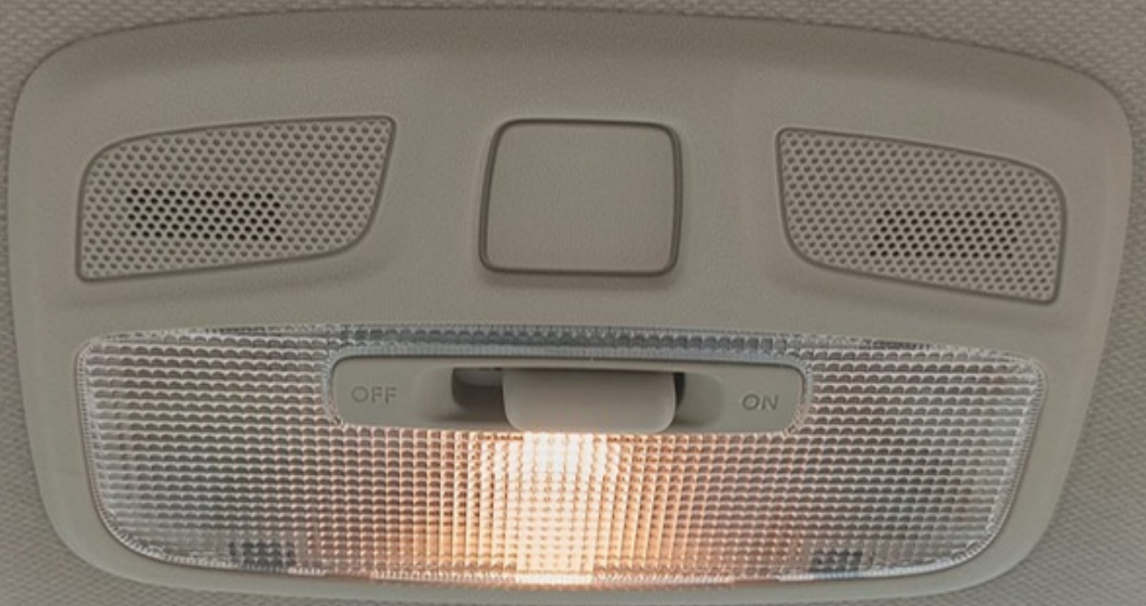
Front Side Roof Light Working
